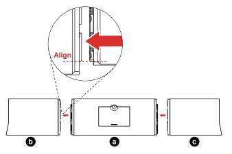
2. Fasten the locks by pushing the hood leaf • in the direction of the arrow as indicated in Picture •, until the hooks are tightly locked in place. Repeat the same procedure to set up the other hood leaf •.
