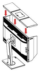
8. Shading hood installation complete.
