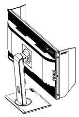
7. Put down top shield and fix on the head.
