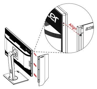
5. Use screwdriver or coin to fasten screw and fix door on the head.
